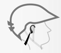
Vibrating disk in ear gear resting on the mastoid process (bone behind your earlobe) warns user of approaching traffic.
